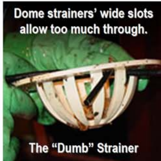
Dome strainers don't work
