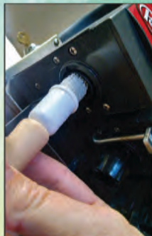
Put Brush Inside Valve Hole
