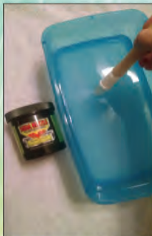
Dip Brush In Soda Nozzle Defender
