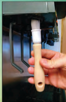
Twist And Turn Inside Valve Hole
