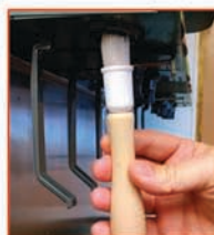
Put Brush inside valve hole. Twist and Turn.
