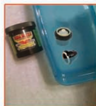
Let nozzles soak 3-4 hours (or overnight), rinse and re-install
