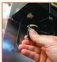
Remove Nozzles & Diffusers From Valve System
