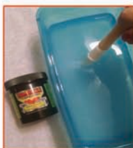
Dip Brush in Soda Nozzle Defender water mixture
